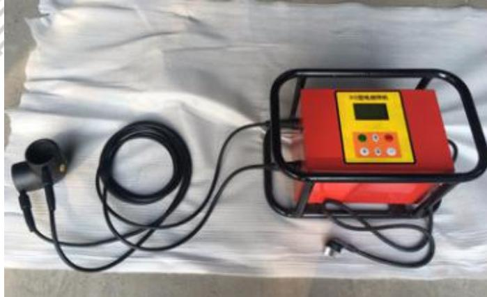
A photograph of an electric fusion splicer for pipe fittings. It features a red and yellow control unit with a digital display and several buttons, connected by a cable to a black probe or electrode. |
