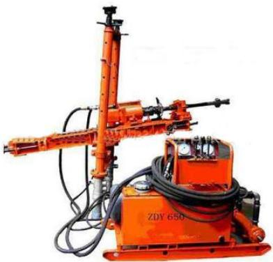
A photograph of an orange hydraulic drilling rig. The rig consists of a vertical mast mounted on a base unit. The base unit features a hydraulic pump unit with a motor and various control components. Cables and hoses are visible connecting the mast to the base. The rig is designed for stationary or semi-stationary operations, such as in a trench or on a flat surface. |
